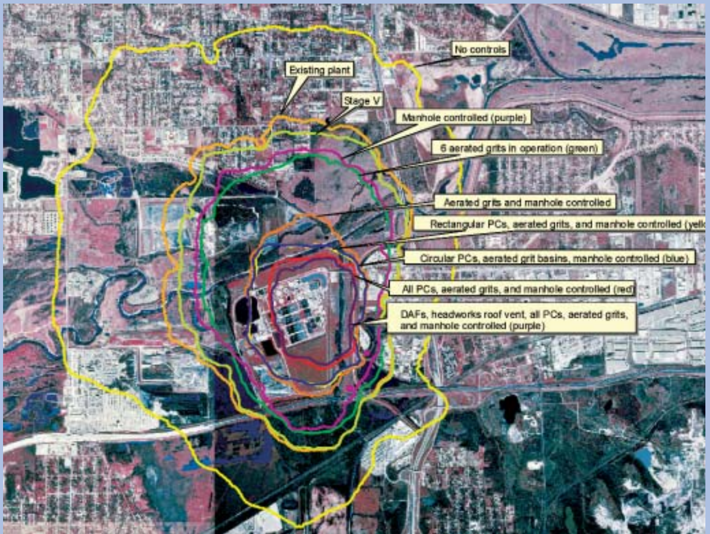
Dispersion model showing effectiveness of CRWS' odor control projects at the system's plant. The CRWS wastewater treatment plant is seen at the center of colored circles. CRWS was developed in the late 1950s when much of the geographic area surrounding the plant was undeveloped. As the area filled in with commercial and residential development, CRWS took a pro-active, good neighbor approach to controlling odors at the plant. With the new superoxygenation technology, odors will be contained within the plant boundaries.
