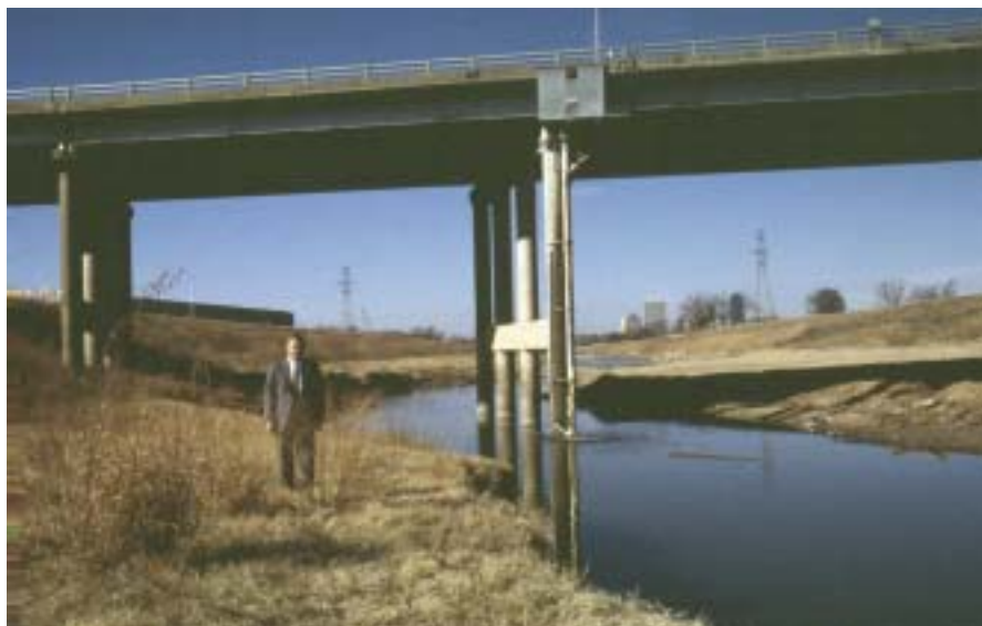
Dr. Browning, TRA's Senior Manager, Planning & Environmental Management, stands next to the Beach Street USGS Gage on the West Fork of the Trinity River. USGS gages produce valuable data for water managers, emergency management personnel, recreational users and environmental monitoring.
