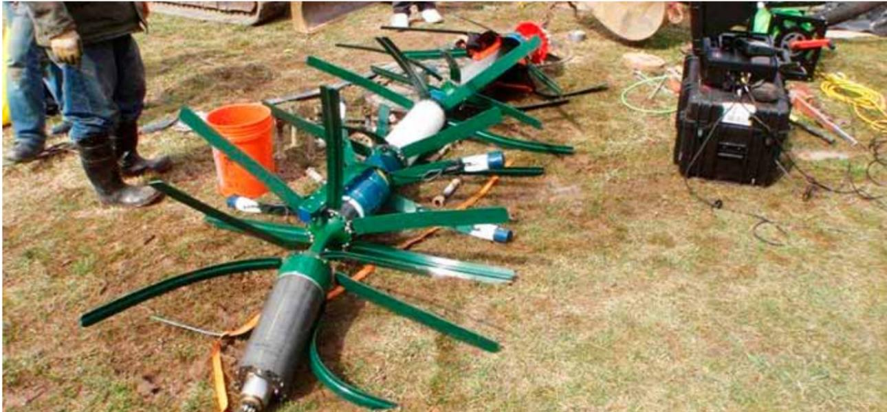
*The Pipediver™, shown here, has yielded preliminary data revealing areas where TRA may need to repair or rehabilitate sections of a pipeline that carries raw water from Lake Arlington to the TCWSP treatment facility.*
